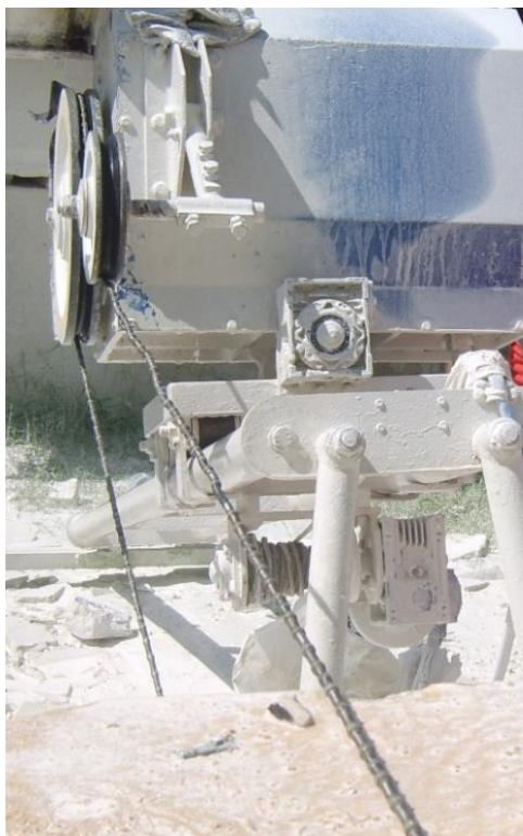
Gambar 7. Diamond Wire Sawing
