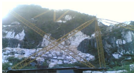
Gambar 1. Metode Quarry , Tipe Side Hill
