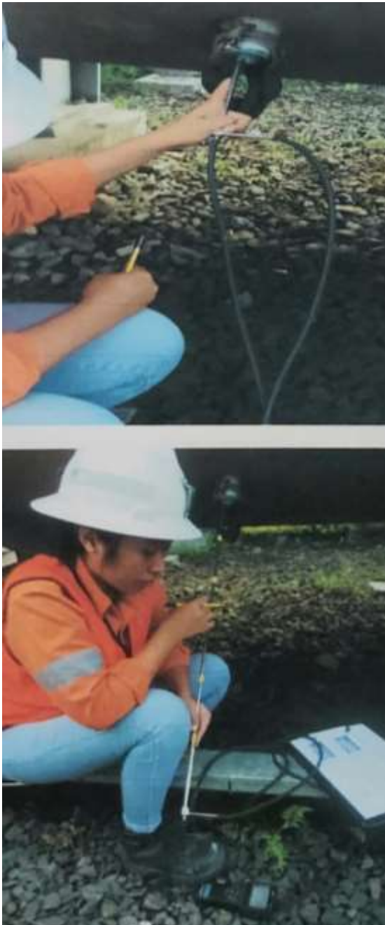
Gambar 2. Pengukuran velocity pressure
