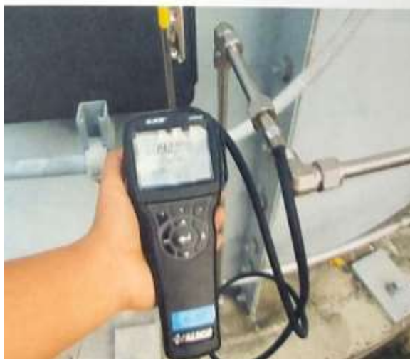
Gambar 4. Pengukuran collar pressure
